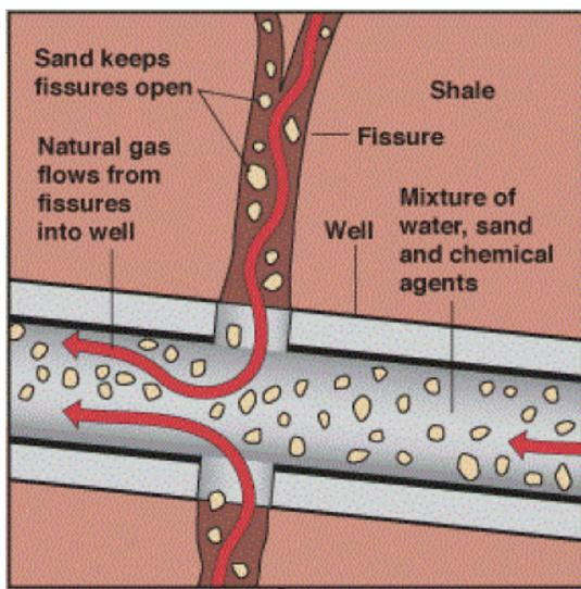
Figure 3. Fracturing the Rock Layer [11]
