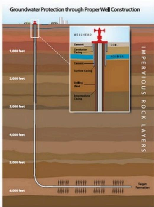
Figure 2. Hydraulic Fracturing/Horizontal Drilling Process [9]
