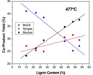
**Figure 9** Co-product yield versus feedstock lignin content at 477°C. Data from [6].
